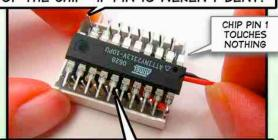
ON THIS SIDE, ALL CHIP PINS- EXCEPT PIN 20-REST AGAINST PINS OF THE LED DISPLAY
